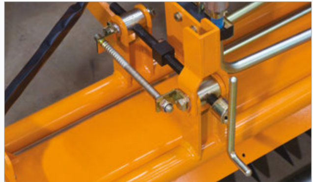
Micro adjusters for depth setting
