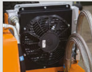
Integral heavy duty Oil cooler
