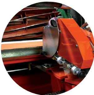
Auto-index allows for unattended automatic relief grinding
