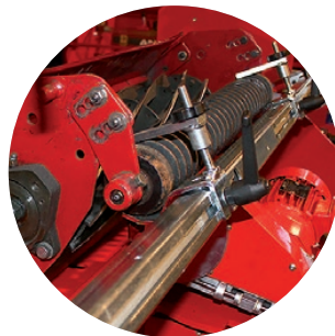
Multi-alignment points facilitates fast and simple reel alignment
